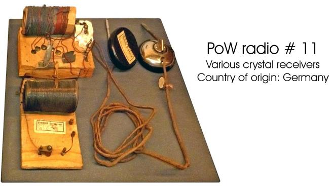
Crystal receiver #1 (top) had a tapped coil and #2 (bottom) a coil with slider.
