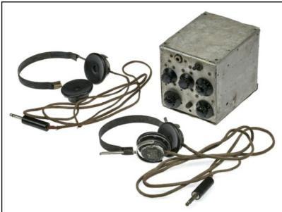
The radio was constructed from aluminium sheet and scavenged parts. Mounted at the front were five black Bakelite control knobs, an on/off switch and a single headphone jack. Located at the rear were terminals for aerial, earth and wires to the power source.
