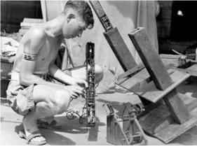
Constructed by Lieut R.F. Wright in Changi Gaol camp was another radio receiver installed in legs of a table (left).
