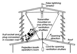
The transmitter was concealed on top of one of the two ventilation shutters in the air duct.
