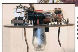
Side view of the receiver showing the round Paxolin breadboard and the two valves (left).
