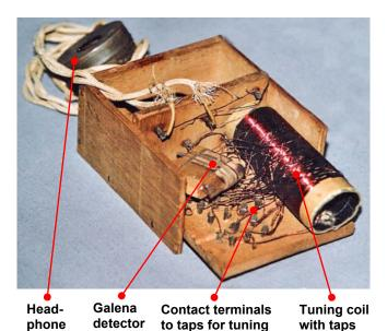
Construction details of the Zeithain 'Gelina' radio. A large number of taps on a coil and two movable plugs provided a rudimentary tuning and adaption of the aerial. The wood, cardboard and string object at the left of the tuning coil was the galena detector. The earphone was constructed using an empty polish tin.
