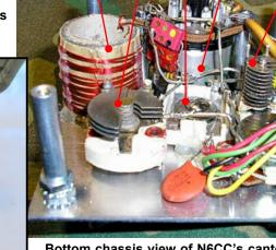
Bottom chassis view of N6CC's canteen radio. (above) For main tuning a mica compression trimmer (C1) was used, adjustable by a screwdriver. Fine tuning (C2) and aerial coupling (C3) was accomplished by two small variable condensers. The coil was wound on a piece of 1-inch bamboo.
