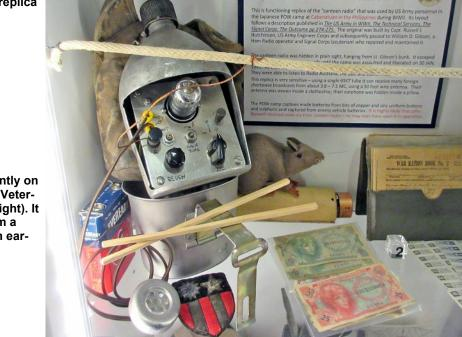
The replica built by N6CC is currently on permanent display at Danville CA Veterans Memorial Building Museum (right). It utilizes a "captured" earpiece from a common telephone handset for an earphone.
